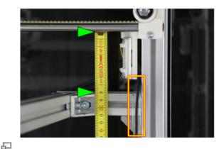
Make sure that the supply lines are running in front of the mounting arm and that it is mounted in the correct height.
