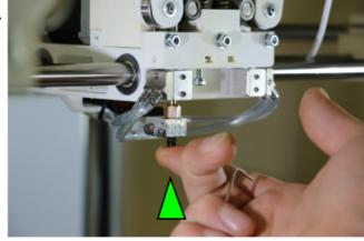
Push the barrel up to the limit and refasten one set screw
