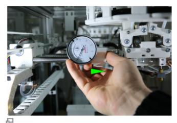
Installing the dial gage at the X-axis.
