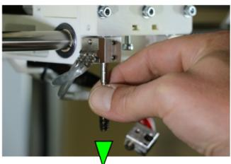
Pull the barrel out of its seat.
