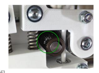
Filament abrasion at the drive gear due to slipping.
