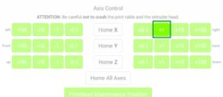
Move the print head to the right to tension the timing belt and zero the dial gage.
