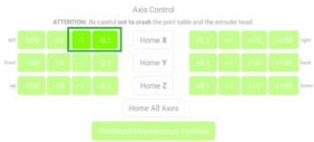
Move the print head against the dial gage's measuring tip.
