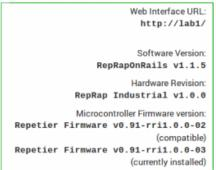
Please send all system information of the GUI's Setup menu: software version, compatible hardware revision, microcontroller firmware version (compatible and current).
