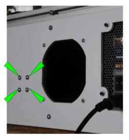
Holding screws of cooling water pump.
