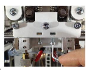
Adjusting the idler lever preload.
