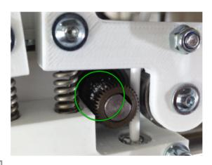
Filament abrasion at the drive gear due to slipping.
