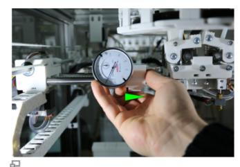
Installing the dial gage at the X-axis.
