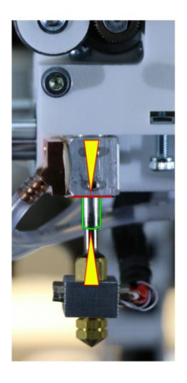
Barrel too low in its seat (exaggerated).
