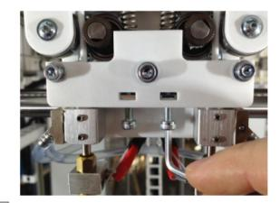
Adjusting the idler lever preload.
