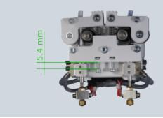
Too high tension of the idler lever spring may result in the gear drive to slip and grind into the filament. Too low tension of the idler lever spring may result in slipping of the gear drive. In both cases the print will abort due to insufficient material transport.
