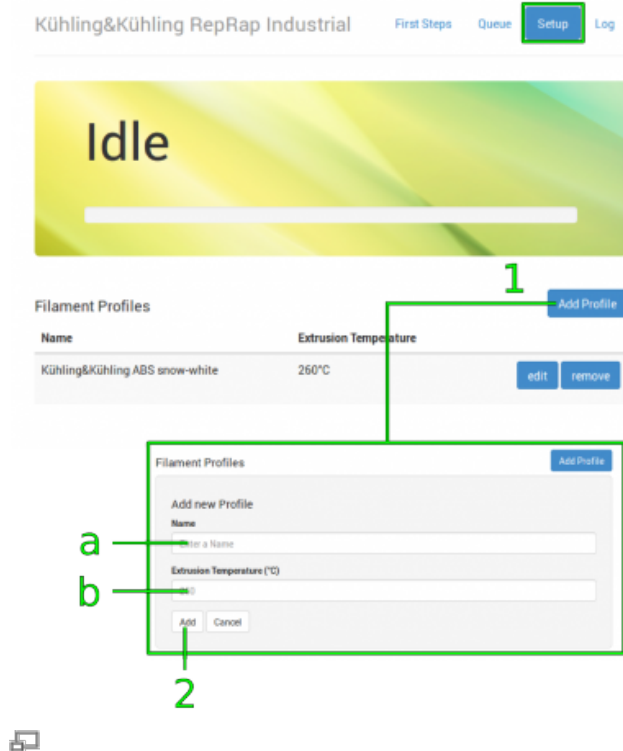
Filament profile setup via the web interface.
