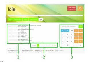
The log screen provides additional information about sent and received G-code commands and the possibility of directly influencing the 3D printer via G-code command input.
