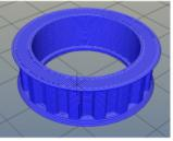
A 3D model in its states during preparation for 3D printing: top-left - the model preview in the 3D modeling software (view taken with OpenSCAD), top-right - the triangulated mesh after .stl-export (view taken with MeshLab), bottom-middle - the G-code preview after slicing shows the single layers calculated by Slic3r (view taken with Repetier-Host).
