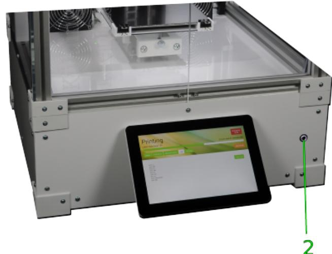
⌚ Waking the 3D printer from standby.
