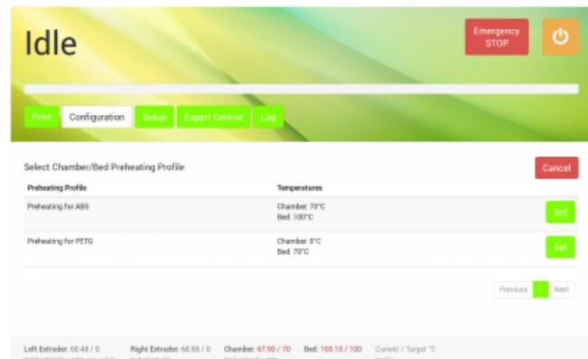
The list of filament temperature profiles of the configuration menu. More profiles can be added via the web-interface.
