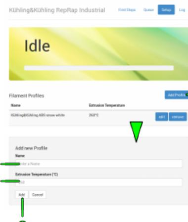
Filament profile setup via the web interface.
