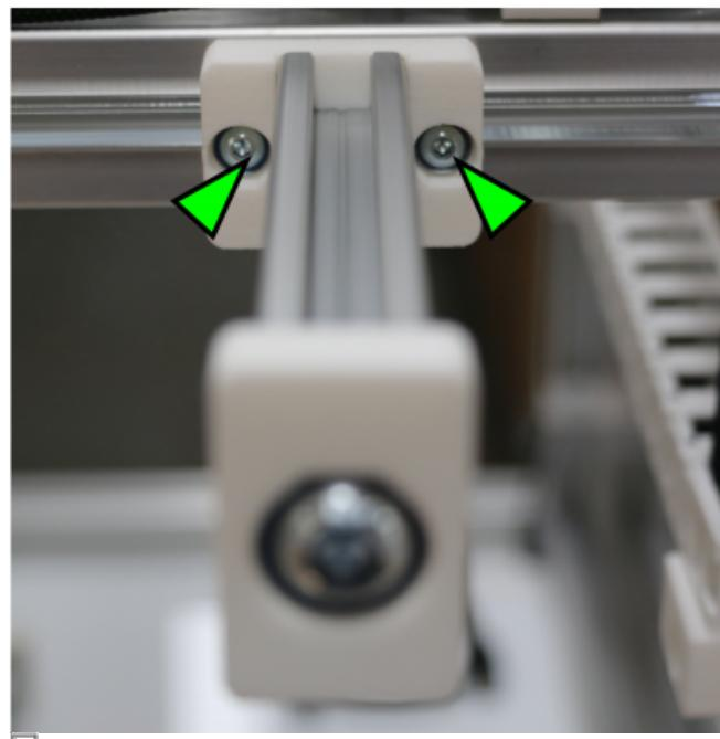
Loosening the fixing screws of spool carriers.
