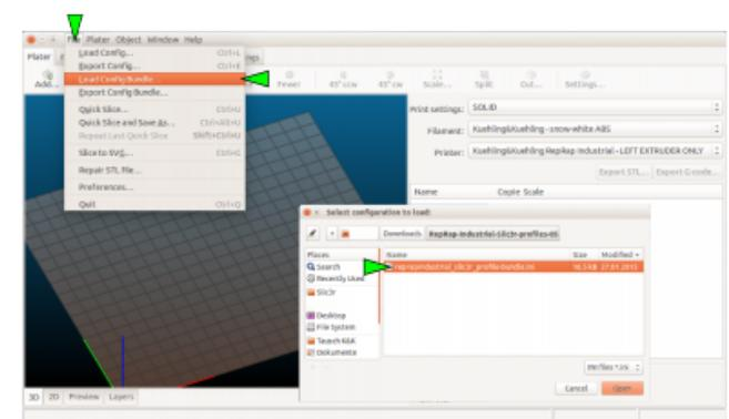
After importing the profile bundles Slic3r is equipped with all necessary presets and ready for operation with the RepRap Industrial 3D printer.
