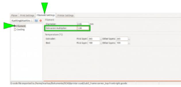
Setting the extrusion multiplier in Slic3r.
