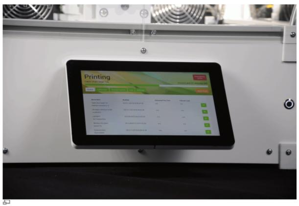
The high-resolution 10"-TFT touchscreen mounted at the front panel enables direct operation of the RepRap Industrial.
