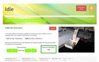
The extrusion multiplier is calculated automatically from the measurement and must be saved in the filament profile of the slicing software.
