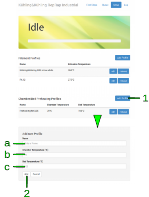
Preheating profile setup via the web interface.
