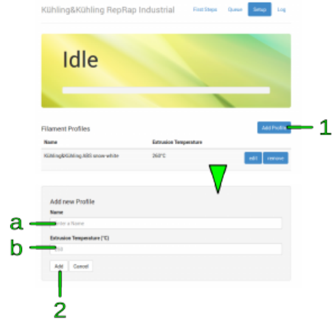
Filament profile setup via the web interface.
