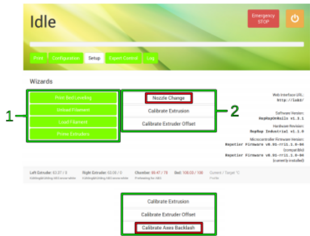
GUI v1.1.0 Setup main screen with wizard selection and system information.
