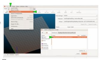
After importing the profile bundles Slic3r is equipped with all necessary presets and ready for operation with the RepRap Industrial 3D
