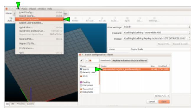
After importing the profile bundles Slic3r is equipped with all necessary presets and ready for operation with the RepRap Industrial 3D
