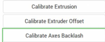
GUI v1.3.0 Setup main screen: the nozzle change wizard was replaced by the backlash calibration wizard.
