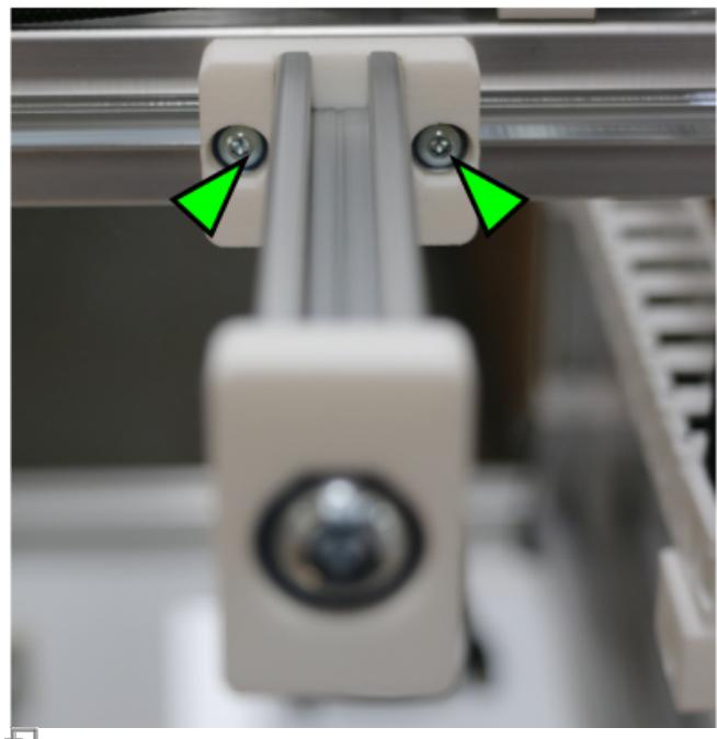
Loosening the fixing screws of spool carriers.
