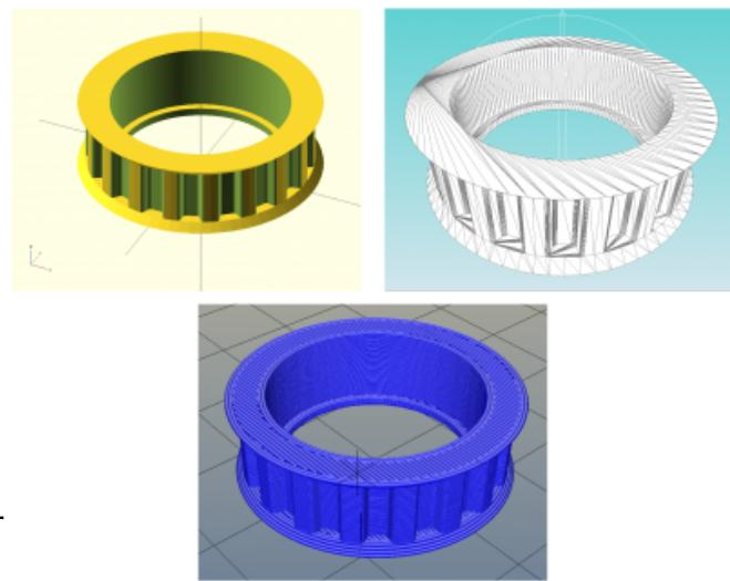
A 3D model in its states during preparation for 3D printing: top-left - the model preview in the 3D modeling software (view taken with OpenSCAD), top-right - the triangulated mesh after .stl-export (view taken with MeshLab), bottom-middle - the G-code preview after slicing shows the single layers calculated by Slic3r (view taken with Repetier-Host).
