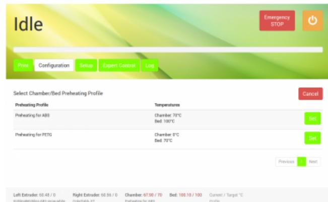
The selected profiles are displayed in the footer of every screen in the order *Current* and *Target* (= set) temperature. While aiming for a target temperature, both values are highlighted red. When displayed gray, the temperature value is either not set or currently not triggered.
