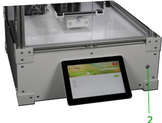
⌚ Waking the 3D printer from standby.
