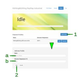
Filament profile setup via the web interface.
