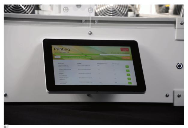
The high-resolution 10"-TFT touchscreen mounted at the front panel enables direct operation of the RepRap Industrial.
