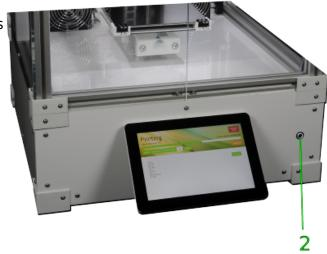
Waking the 3D printer from standby.
