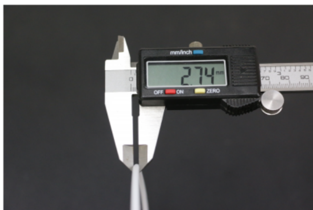
Third measured diameter - this filament exceeds the stated tolerance and must be replaced.
