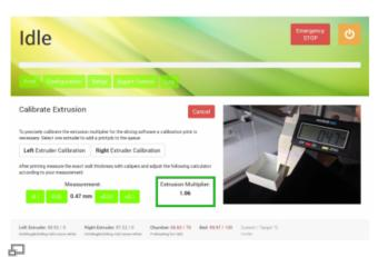
Adjust the preset "0.50 mm" value via the touch buttons and read the necessary extrusion multiplier directly from the display.
