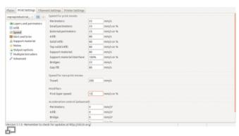
Slic3r Print Settings - setting the first layer extrusion speed
