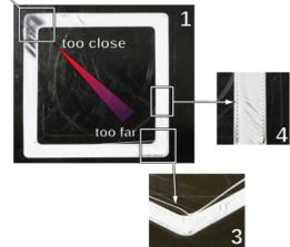
Leveling mistakes: examples of characteristic appearances of the first layer.
