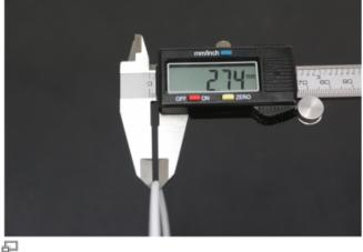
The measured diameter is below the admissible tolerance ...
