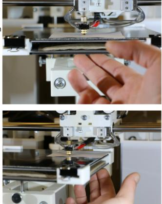
Manual leveling with paper spacer - front and hind right leveling point.
