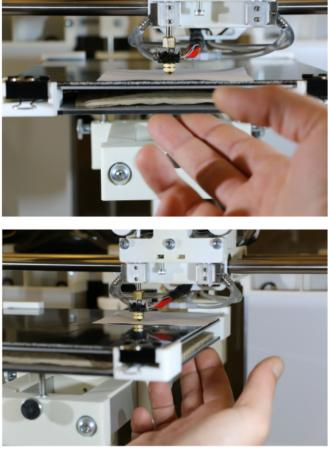
Manual leveling with paper spacer - front and hind right leveling point.
