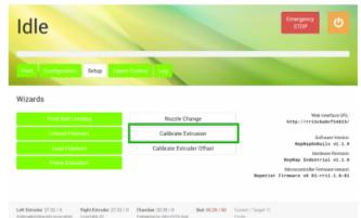
Choose the [Calibrate Extrusion] wizard from the Setup menu (either software version).
