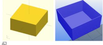
The 30x30x15 mm calibration cube as OpenSCAD model and ready sliced with Slic3r (view taken with Repetier-Host).
