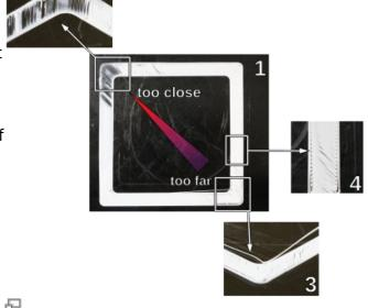
Leveling mistakes: examples of characteristic appearances of the first layer.
