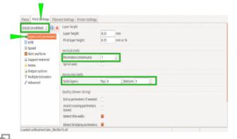
Select the *Layers and perimeters* according to the adjacent table.
