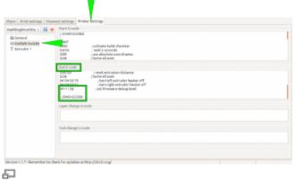
Switching off the build chamber heating
