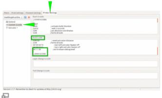
Switching off the build chamber heating elements by modifying the Slic3r custom End G-code.
