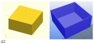
The 30x30x15 mm calibration cube as OpenSCAD model and ready sliced with Slic3r (view taken with Repetier-Host).
