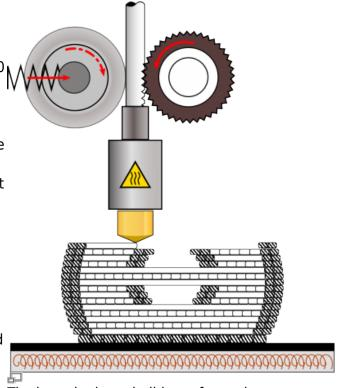
The layer-by-layer build-up of complex geometries becomes possible with FFF additive manufacturing machines.
