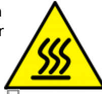
Hot surface warning sign.
