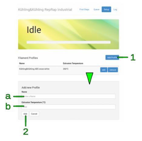
Filament profile setup via the web interface.
