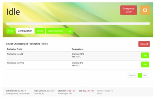
The list of filament temperature profiles of the configuration menu. More profiles can be added via the web-interface.
