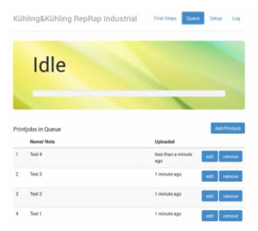
The Queue contains list of uploaded print jobs in a top-down order with the last upload first.
