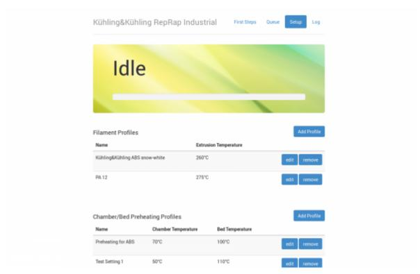
Temperature profiles on the *Setup* screen of the web interface.
