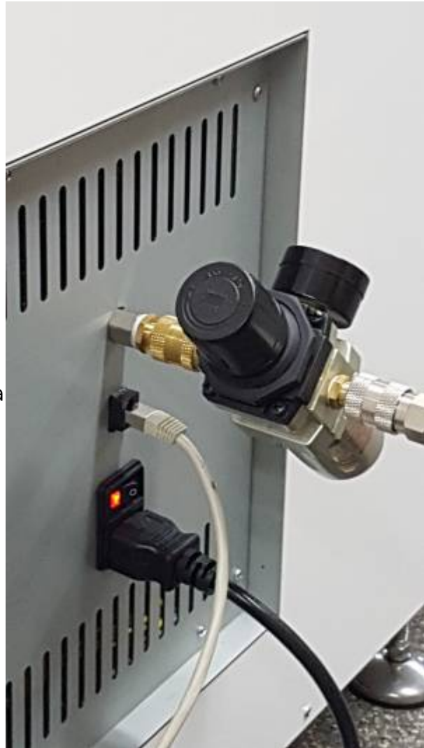
Connections on the rear side of the machine: 230 V power plug, RJ45 Ethernet socket and DN 7.2 pressure reducer.
