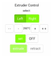
This new feature was installed to give you the opportunity of finding the correct extrusion temperature of any material more directly and comfortably without having to use the [Prime Extruders] wizard.
