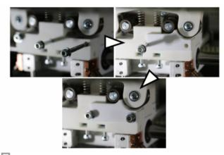
Installing the adapter for flexible filaments.
