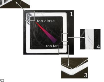
Leveling mistakes: examples of characteristic appearances of the first layer.
