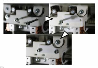
Installing the adapter for flexible filaments.
