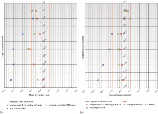
The deviation decreases significantly when the thermal expansion is compensated.
