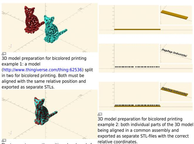
The two parts correctly positioned and ready for export.
