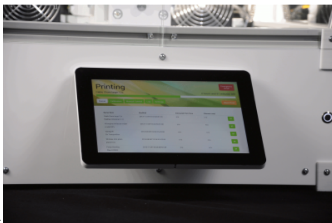
The high-resolution 10"-TFT touchscreen mounted at the front panel enables direct operation of the HT500.
