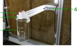
The wiper makes sure that the nozzle tip is always clean and well filled after a tool change
