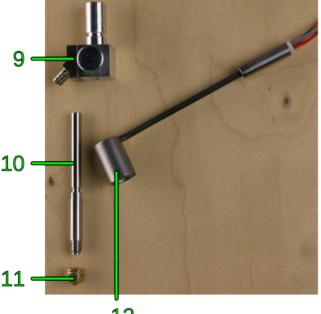
The nozzle is exchangeable to provide different bore diameters for different materials, layer thicknesses or print speed. Ex factory, the 0.35mm tip is preinstalled. Additionally, three nozzles with diameters of 0.25mm, 0.5mm and 0.75mm are included. The tips are distinguishable by the engraved markings.
