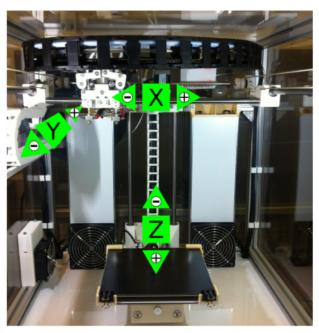
Denotation and direction determination of the axes.
