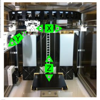
Denotation and direction determination of the axes.
