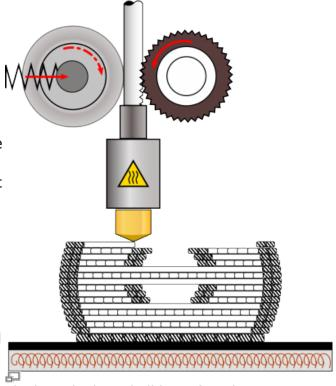
The layer-by-layer build-up of random geometries becomes possible with FFF-3D Printers.
