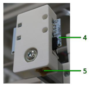
ㅋ Filament inlet with limit switch and dust wiping sponge.
