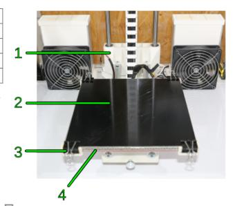
Print table and print bed fastened with four bulldog clamps
