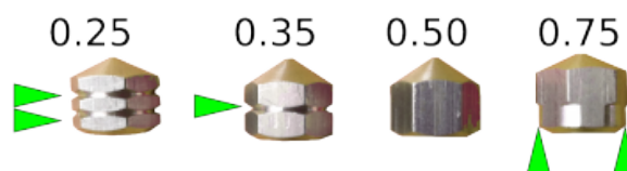
Markings to distinguish nozzle sizes.
