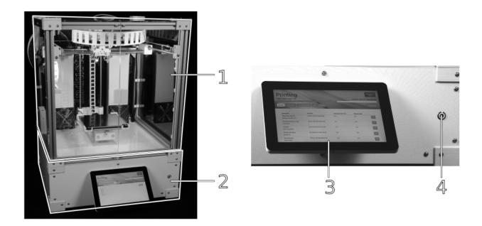
The two main functional sections of the HT500 HMI touchscreen for direct operation and wake 3D Printer: the build chamber with the functional button at the front panel. components and the electronic chamber containing the regulation electronics.
