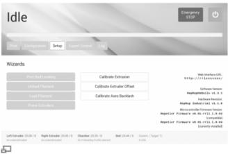
The web interface URL on the SETUP screen is required for connecting the 3D Printer with your local network.
