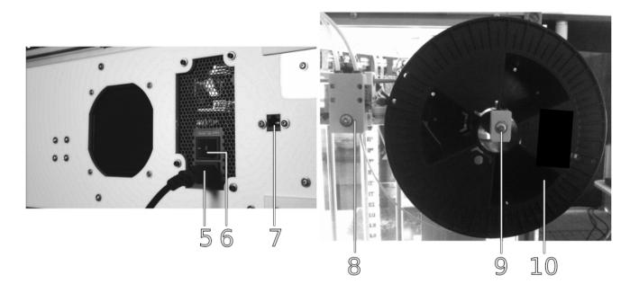
Power/network connections and mains switch at Filament feed system at the rear of the build the rear panel.
