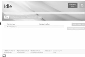
After the boot sequence the operating screen starts with the PRINT tab in IDLE mode. At initial commissioning, the print-job queue is empty and no temperature profiles are selected.
