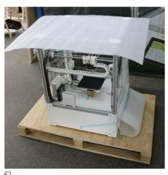
Place the 3D Printer in the middle of the pallet and cover it with foam foil.
