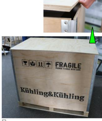
Ensure the lid fits so that tensioning the lashing straps will work.
