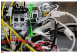
Bridge the pins with a jumper to activate the chip's programming mode.
