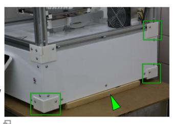
Reinstall in reverse order, remove the wood and Lift the 3D printer at one side; the feet and the hind cover angle must be removed.
