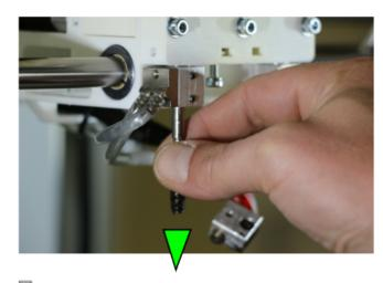
Pull the barrel out of its seat.
