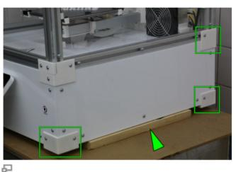
Reinstall in reverse order, remove the wood and Lift the 3D Printer at one side; the feet and the hind cover angle must be removed.
