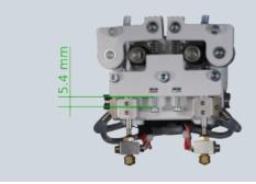
Too high tension of the idler lever spring may result in the gear drive to slip and grind into the filament. Too low tension of the idler lever spring may result in slipping of the gear drive. In both cases the print will abort due to insufficient material transport.
