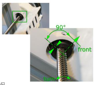
Align the recess of the clamp collar parallel to the 3D Printer's front.
