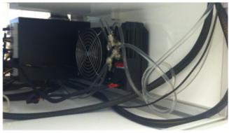
Cooling water pump mounted in the electronic ir.chamber.
