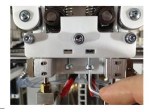
Adjusting the idler lever preload.
