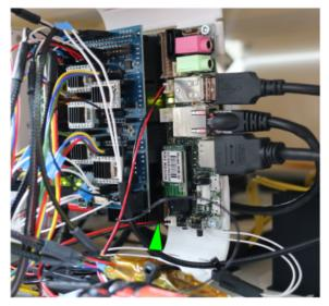
SD card slot at the lower edge of the UDOO board behind the dissipator.
