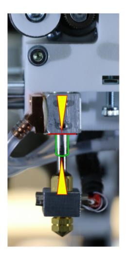
Barrel too low in its seat (exaggerated).
