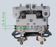
Too high tension of the idler lever spring may result in the gear drive to slip and grind into the filament. Too low tension of the idler lever spring may result in slipping of the gear drive. In both cases the print will abort due to insufficient material transport.
