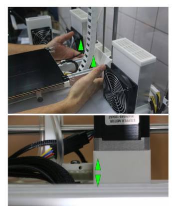
Try to lift the Z-elevator and watch the pulley. If the pulley moves up and down, the clamp collar must be repositioned.
