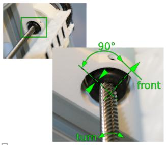
Align the recess of the clamp collar parallel to the 3D Printer's front.
