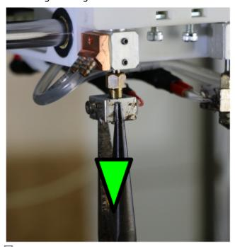
Pulling the heating block off the barrel.
