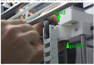
Hold down the pulley and push up the clamp collar.
