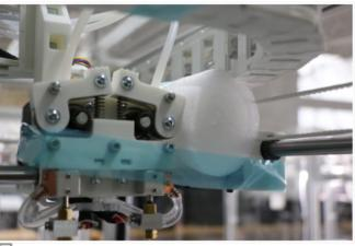
Cushion the extruder head with the foam coil against the right carriage and tightly fasten it with tape.
