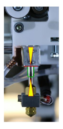
Barrel too low in its seat (exaggerated).
