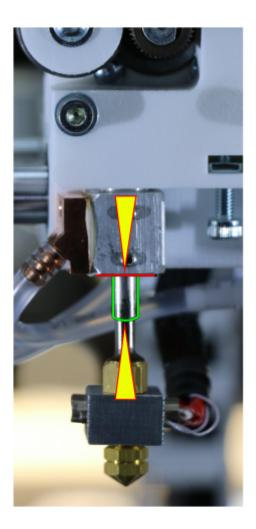
Barrel too low in its seat (exaggerated).
