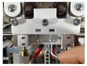
Adjusting the idler lever preload.
